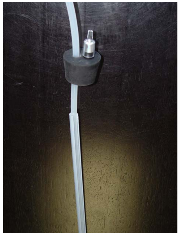
Figure 3. Pickup tube passing through rubber stopper, with check valve.
