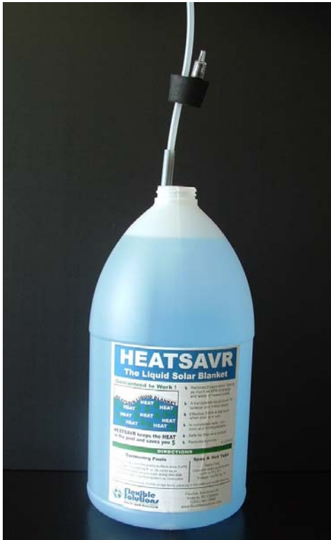
Figure 5. Heatsavr Suction Tubing (uptake side) with Standpipe in Heatsavr Jug
